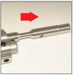
**Stage 2**Remove the main bolt from Inferno, (Part No.0045) should slide out esaily.
