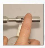
**Stage 4**Using Inferno lube squirt a few drops on the long bolt.
