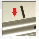
**Stage 6**Push the cocking handle back into the long bolt. The knurled part should be facing up. It should click into place.
